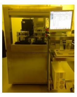
The Rainbow TCP 9600 Standalone System is a single wafer, vacuum load-locked low pressure metal etch system. Semigroup Equipment Sales provides a customized (to your specifications) totally refurbished Rainbow TCP 9600 Metal Etch Plasma Reactor that is fully tested at our facility. Upgrades included are wafer size conversions, (150mm, 200mm etc.) Electrostatic Chuck Upgrades, Computer Upgrades and more.
